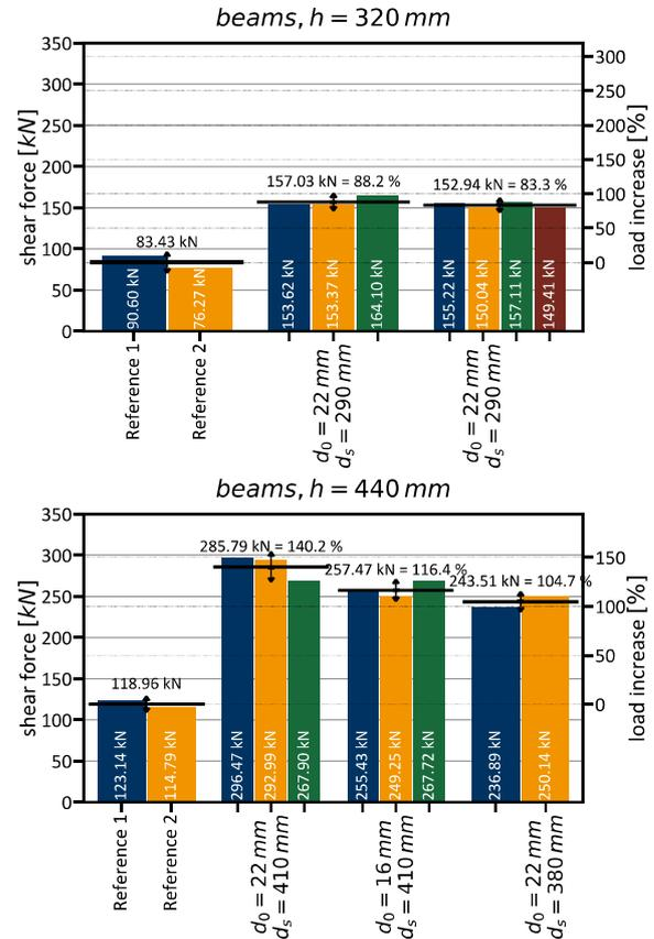
Figure 3. Failure loads of tests with concrete beams with two different heights and screws with variable diameter and installation depth
