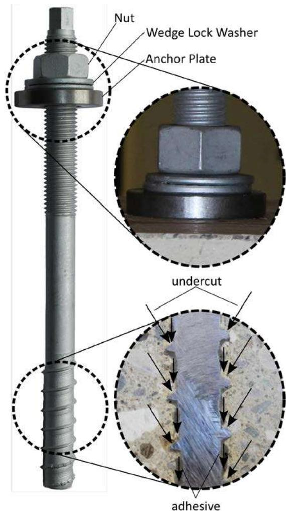
Figure 1. Adhesive Concrete Screw Anchors with load transfer mechanism and bracing
