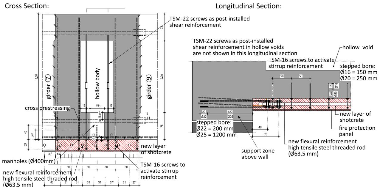
Figure 6. Planned strengthening system of segment 34 with concrete screws as post-installed shear reinforcement and threaded rods of high strength steel as bending reinforcement in a new shotcrete layer
