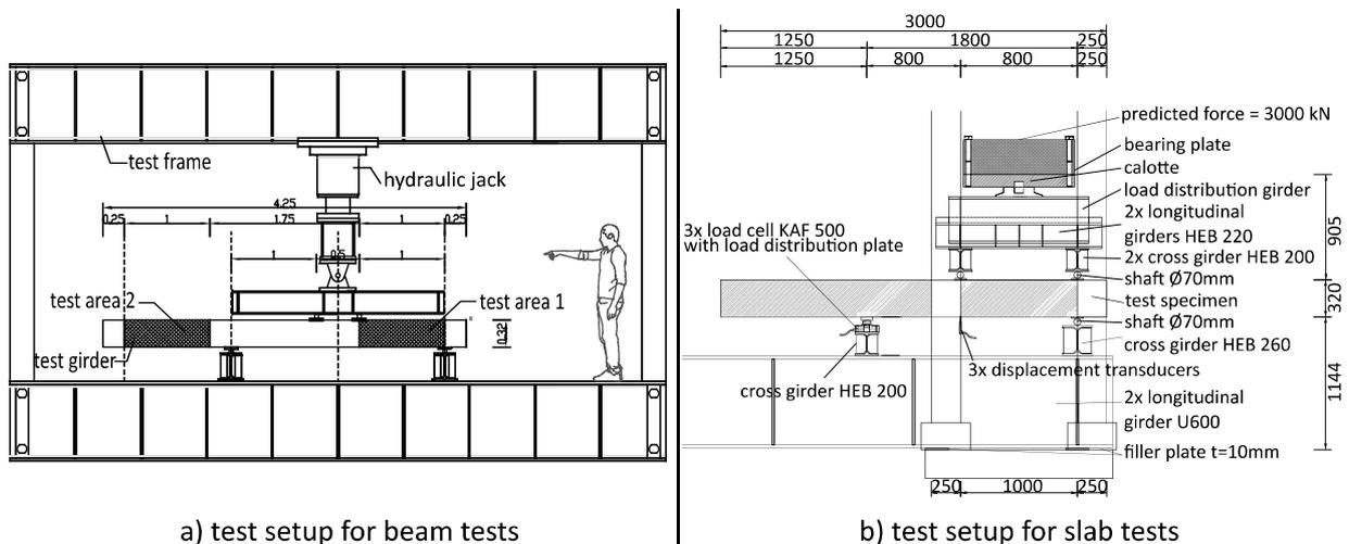
Figure 2. Test setup for beam tests at the University of Innsbruck and for slab tests at the University of the German Federal Armed Forces Munich
