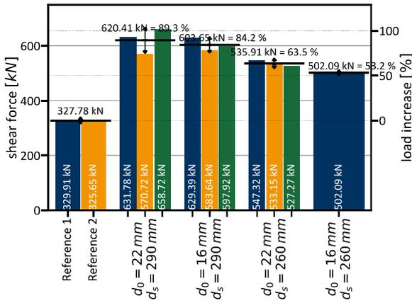
Figure 4. Failure loads of tests with concrete slabs and screws with variable diameter and installation depth
