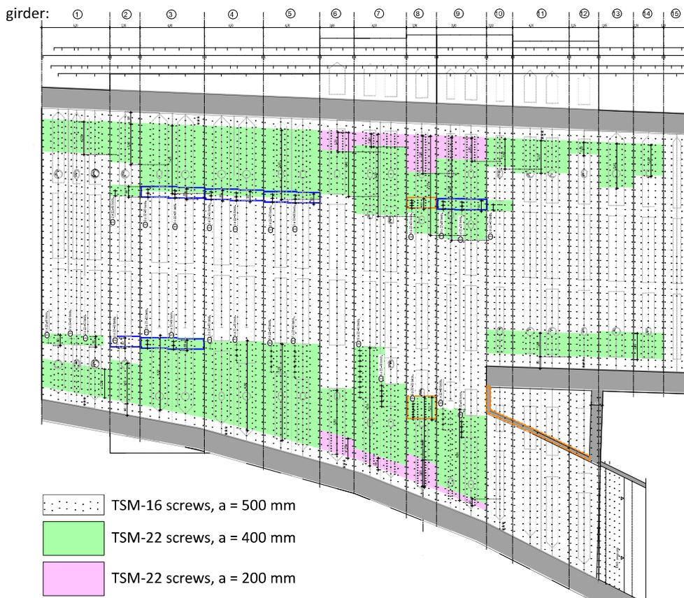
Figure 7. Plan view of section 34 with south exit and different areas shear strengthening
