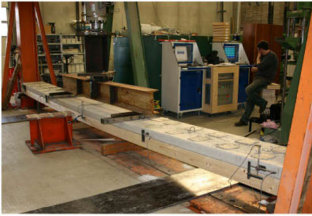
Figure 3. Bending test with cams as shear connectors.
